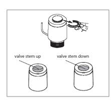
The actuator is equipped with a visual position indicator to show when the actuator position is either open or closed. The inner black cover located on the top of the actuator will project above the white enclosure when the valve is open. When the inner black cover is flush with the white enclosure, the valve stem is down and seat of the valve is closed.
