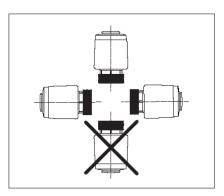
The actuator's orientation should be mounted in either a horizontal or vertically up position. The base ring of the actuator should be tightened by hand.
